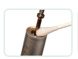
1b. Dip a cotton swab in Isopropyl alcohol or a pH neutral solution or detergent and clean around the inner contact ring until
