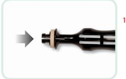
1b. Place a large rubber ring on the Hand Piece Cleaning Tool
