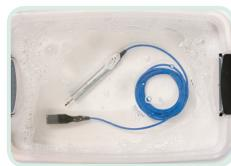
1a. Immerse Hand Piece in pH neutral detergent or pH neutral enzymatic detergent for up to one hour and clean with a soft bristle brush or equivalent.
