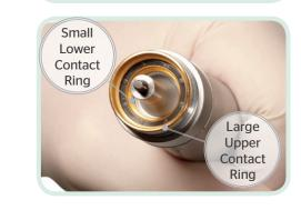
Note: Please be sure to clean both the smaller lower contact ring and the larger upper contact ring. Repeat as necessary until clean.
