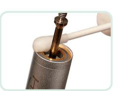
1c. Dip a cotton swab in Isopropyl alcohol or a pH neutral solution or detergent and clean around the outer contact ring until
