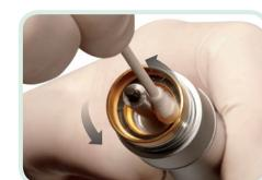
2c. Dip a cotton swab in Isopropyl alcohol or a pH neutral solution or detergent and clean around the inside of the lower contact ring until
